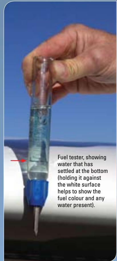
Fuel tester, showing water that has settled at the bottom (holding it against the white surface helps to show the fuel colour and any water present).
