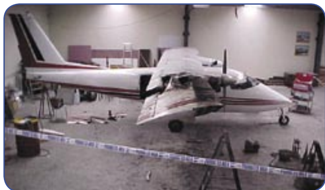
The aircraft was extensively damaged by explosion and fire.
