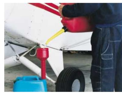
strap, then the current will flow safely from one body to another. However, if there is no conductor, and there is a big enough difference in the electrical potential, then a spark can bridge the gap.
