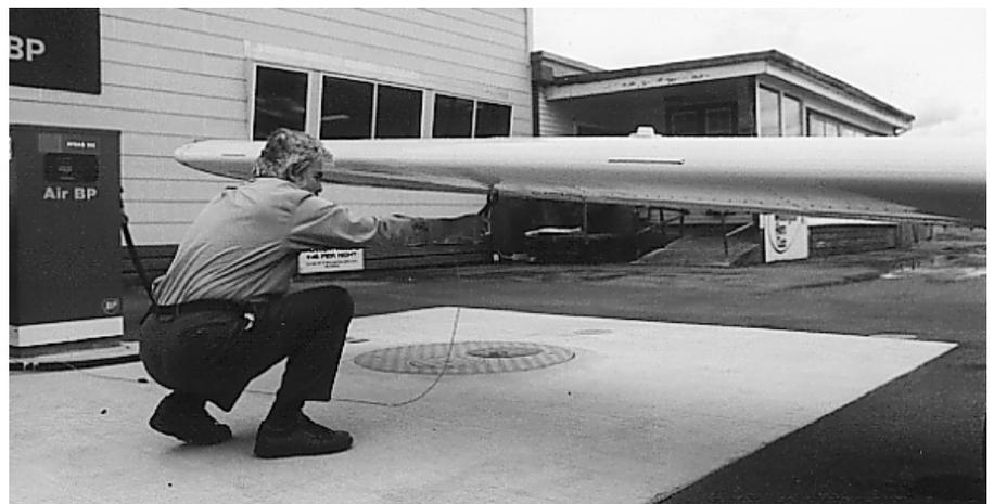
*Securely attaching the bonding wire to a non-painted metallic surface (one that can convey an electrical charge to or from the aircraft fuel tank) before refuelling begins will equalise any potential difference that exists between the aircraft and the fuel pump.*
