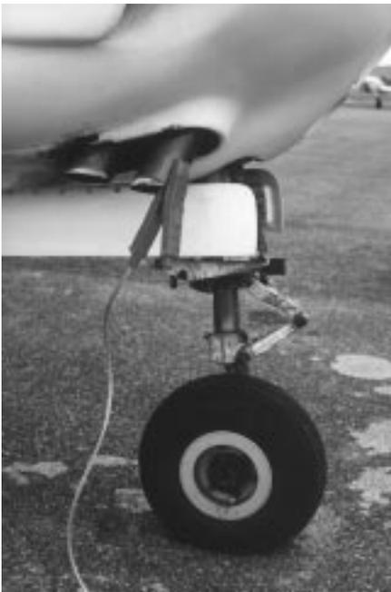
*Ensure that the static line clip makes metal-to-metal contact with the aircraft structure – this may require a slight scraping motion (on a non-painted surface such as an exhaust pipe or undercarriage strut) to confirm that a contact has been made. Note that many aircraft have grounding plug receptacles at or near the fuelling caps, and it is worth utilising these.*
